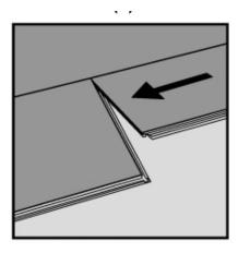
8. Place the panel tight to the short end of the previous panel and fold down in a single action movement.
