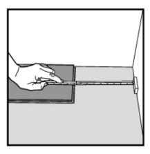
5. If cutting with a jig saw, the laminate surface should be turned down. If cutting with a hand saw, the laminate surface should be face up.
